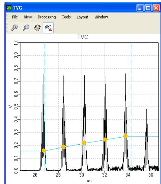
**Figure 4.** TVG distorting A-scan for one purpose.
