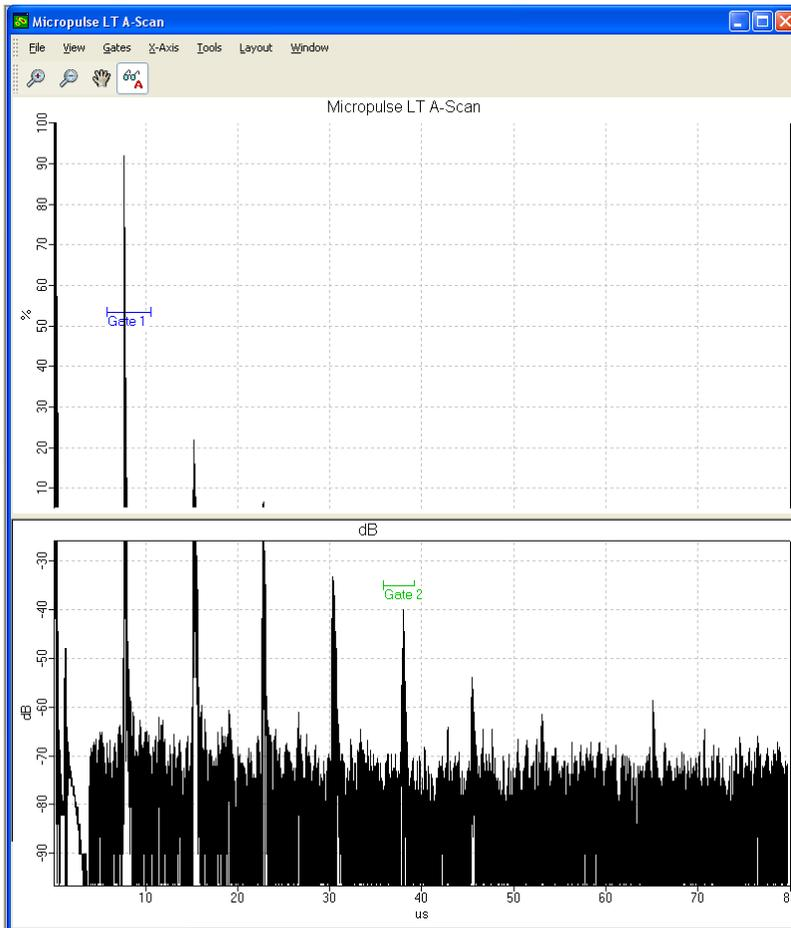
**Figure 6.** A hybrid display showing both linear and log plots.
