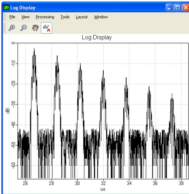
**Figure 3.** Log display showing noise below -40dB (1% FSH).
