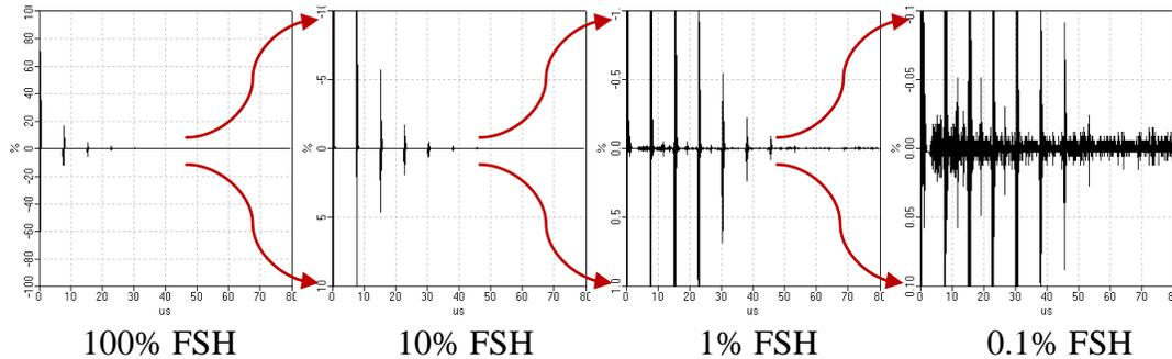
**Figure 5.** Vertical magnification of a wide dynamic range signal.
