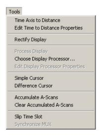
**Time Axis to Distance** Converts the time axis on the A-scan to distance.
