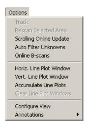
**Track** Provides a crosshair cursor to pick points on a Cscan. The scanner will drive to the picked locations
